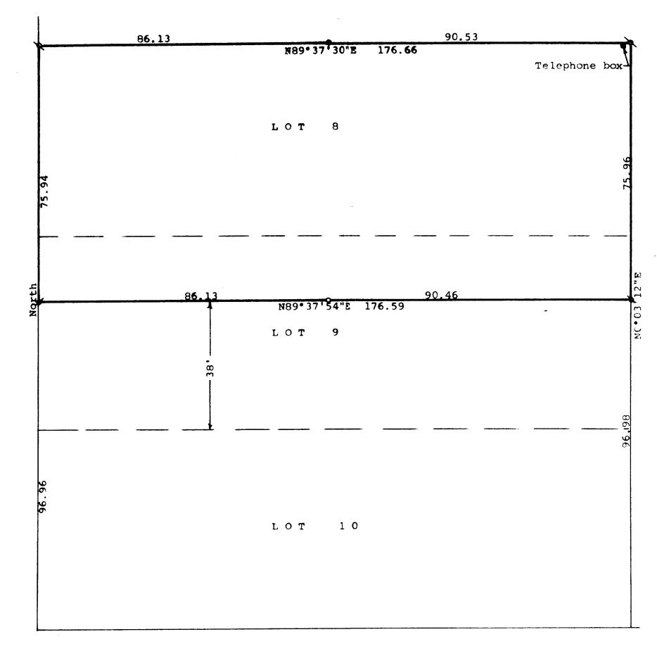
Scale - 1" = 26" □ 3/4" Iron Pipe Found  $0 = \frac{1}{2}$ " X 24" Iron Pipe Set Bearings referenced to the assumed bearing of North along the east line of Seventh Street Survey ordered by: Contury 21, Skandia Realty
